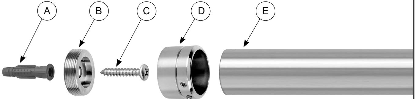
1. Locate and attach Threaded Plug (B) to wall using Wall Anchor (A) and Structural Screw (C)
